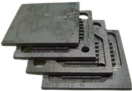
$\text{SiC}_f/\text{SiC}$  plate-type heat exchanger
