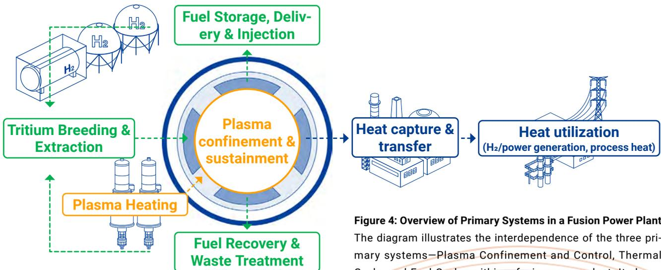
**Figure 4: Overview of Primary Systems in a Fusion Power Plant**
