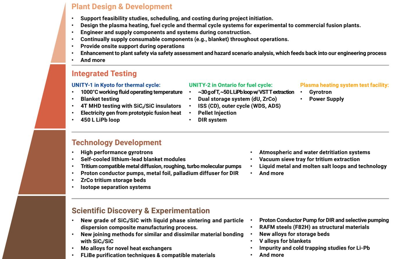
**Figure 2: Kyoto Fusion's Multilevel Approach to Fusion Power Plant Development.**
