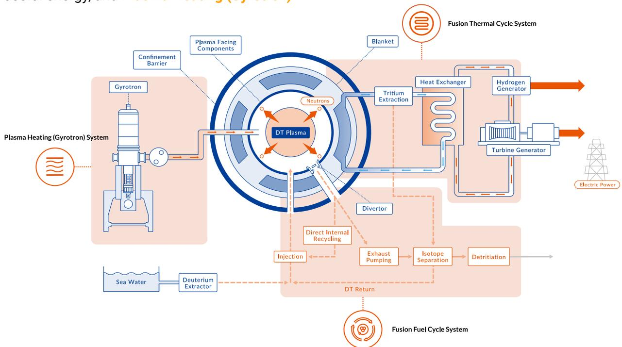
**Figure 1: Conceptual Coupling of Systems Developed by Kyoto Fusioneering**
